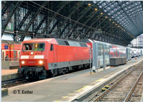
**Prototype:** German Railroad, Inc. (DB AG) fast general-purpose locomotive, road number 120 202-7, with the "Commuter Service Package". Paint scheme as of 2019. B-B wheel arrangement. Built starting in 1987.
