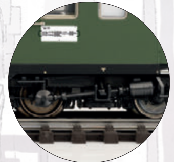
Prototypically equipped with Minden-Deutz (MD) heavy type 330 trucks including a type D 150 cardan axle generator
