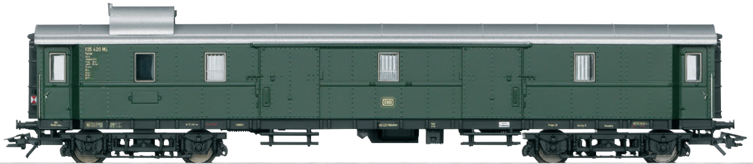
Baggage car includes built-in marker lights and wheel pickups for power supply
