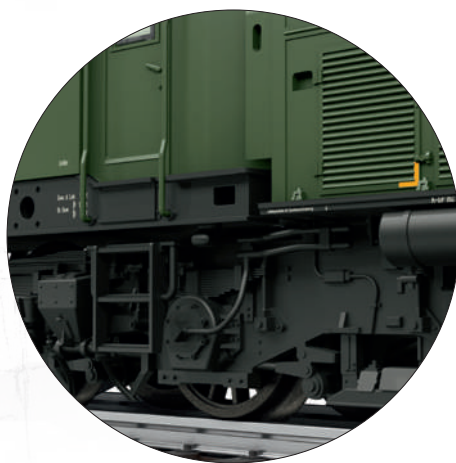
The power truck frames and the approach lamps are executed with precision
