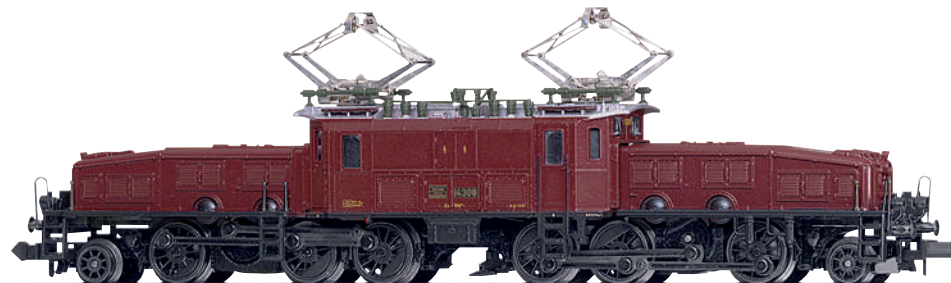
Design with diagonal side rod drive
