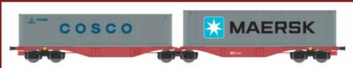
Carro intermodale articolato Tipo Sggrss 80' ČD Cargo con carico di container. Articulated container wagon Type Sggrss 80' of ČD Cargo with container. Gelenk-Containertragwagen Typ Sggrss 80' der ČD Cargo mit Containern.
