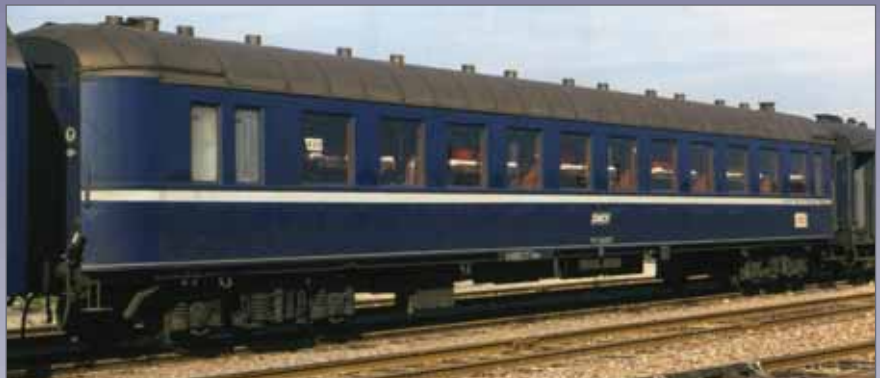
Carrozza letti ex CIWL, Tipo Ub, con bourellets, costruzione Nivelles, livrea Pool TEN e carrelli N2, immatricolata SNCF, ep. IV. Former CIWI sleeping car Type Ub, built by Nivelles, Pool TEN livery with N2 bogies, used by SNCF, ep. IV. ISG Schlafawgen Typ Ub, von Nivelles gebaut in Pool TEN Lackierung mit N2 drehgestellen, von SNC. Ep. IV.
