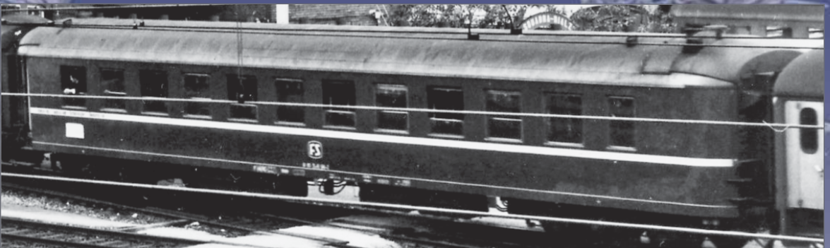
Carrozza letti ex CIWL, Tipo Ub, con bourellets, costruzione Ansaldo, livrea Pool TEN immatricolata FS, ep. IV. Former CIWI sleeping car Type Ub, built by Ansaldo, Pool TEN livery, used by FS, ep. IV. ISG Schlafawgen Typ Ub, von Ansaldo gebaut in Pool TEN Lackierung, . Ep. IV
