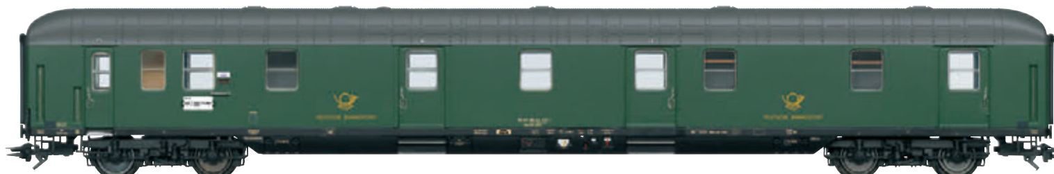
Prototypically equipped with Minden-Deutz (MD) heavy type 330 trucks including a type D 150 cardan axle generator
