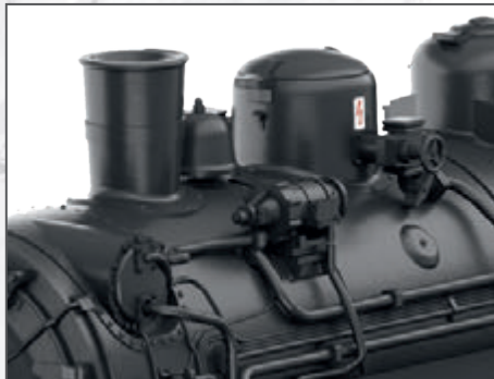
Turbo dynamo for electric lighting and bell between the smoke stack and steam feedwater dome
