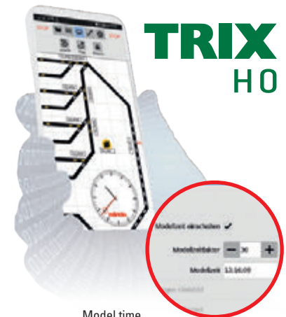
Model time can be added as an element on an accessory controller or a panel. The model time factor can be defined in the settings.
