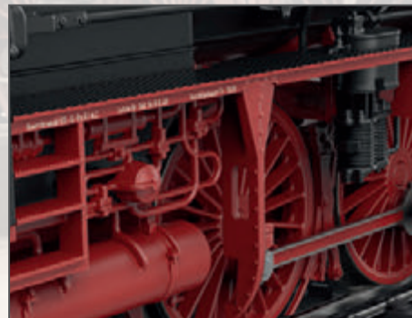
The mechanism for the automatic load-proportional braking system is mounted on the supports for the former streamlining.
