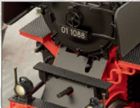
One of the features of the overhaul at Henschel: The smokebox access step does not extend up to the boiler.
