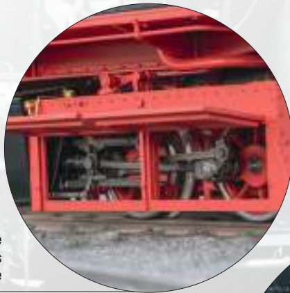
All of the hatches for the truck covers can be raised as in the prototype
