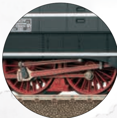
The valve gear and side rods are fully developed, and the streamlining is thin like the prototype
