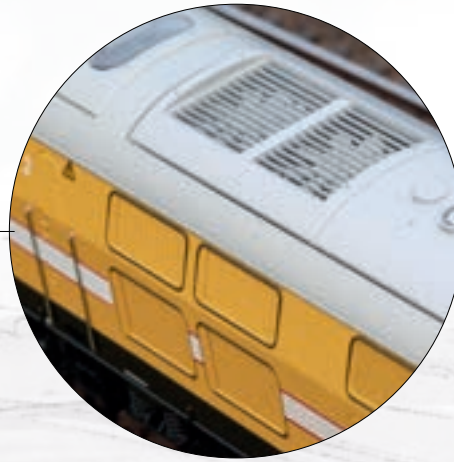
The working ventilation wheels can be controlled digitally in pairs
